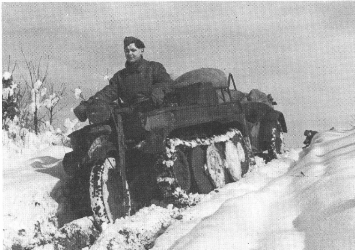
Below Towing a trailer, a Kettenrad makes its way down a well-travelled slope (Maier) (31/2424/29).
